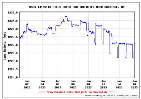
Figure 47. Gauge Height (feet); below Hills Creek Dam PWR - Middle Fork Willamette River
