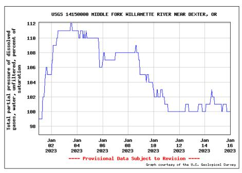
Figure 31. Total Dissolved Gas Saturation (%); Middle Fork Willamette River, Near Dexter, OR
